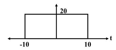
Find the Fourier transform of the above signal and plot the amplitude and phase plot of the signal. Put frequency, f in the  $\times$  axis (not  $\omega$ ).
